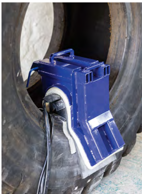
Sistema per talloni / Bead repair system XLBRS (giant OTR 40.00 R57 and 59/85R63)
